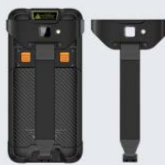
RB-RD66-HS Hand strap with buckle 2 pcs M1.6 screws are necessary.
